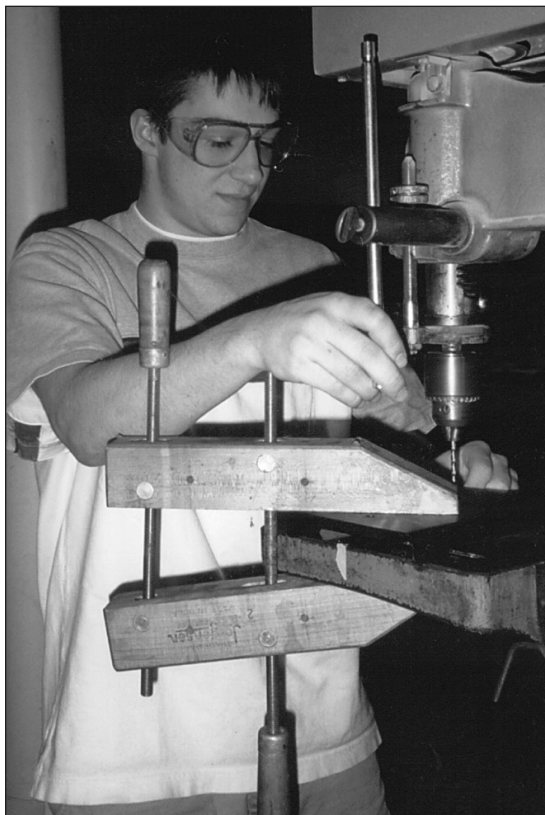
A student drills holes in the metal base.
